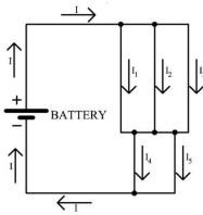
non-compressible and lossless nature makes it like an ideal river of water which may split to branches and recombine. When recombined, all the water of the (ideal) river should have exactly the same flow rate as before the branching. In the circuit on the left, after flowing through the branches, the current becomes
