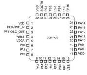
Let's consider a small MCU like the one on the left. It is from ST Microelectronics. ST named any GPIO pin as PXX (P from "port"). We can set any of those in the mode we want (input or output) initially. We can **read** the real time value of each **input** pin, which will be 1 if
