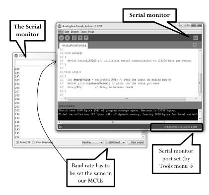
"Serial" is an object already created waiting for us to use it. Serial.println() function prints its parameter as text followed by an "Enter key pressing" to go to a new line. There are more function members of this class, also for reading from your UART if you send information over the serial monitor or from another application or any UART, like receiving data from a GPS device for example.
