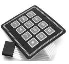
A membrane keypad consisted of many buttons on a flexible and adhesive material about 1mm thick with custom printing on its surface
