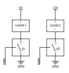
or NPN output switching concept. It is usually the first and best choice too. On the circuit on the left imagine we have such systems (boxes with the switches) **that connect only to the ground** (take that as a limitation and a feature too), they have a
