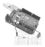
can be, let's see how we can practically connect an LED to it and control it by software (on the left). The photo is accredited to the greatest site for Arduinos, after the www.arduino.cc, the www.adafruit.com website that has flooded the Arduino open source library with its own contributions. (*Credit: Simon Monk, https://learn.adafruit.com/assets/2158*). That job
