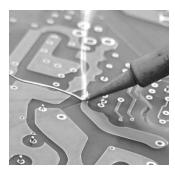
water on the tip of the soldering iron. We move that drop where we should in order to join together wires, pins, copper pads on PCBs etc. (we will come later on those), remove the tip, wait a fraction of a second to cool down and that drop is solid, frozen at the place we left it, holding the parts together. Any smoke coming out is
