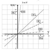
the left  $0.1\Omega$ ,  $1\Omega$ ,  $2\Omega$  and  $10\Omega$  all on the same diagram as to have immediate comparison, we see that the less the resistance the steeper is the slope of the line, the more it is the less is the slope. Let's start from the plot of  $1\Omega$ . Two Volts make 2Amps, 10V make 10A etc.., going higher in resistance, 10V will make less and less Amps up to the point
