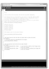
control of the **MCUs** peripherals **CPU** and functionality. They called it That "Wiring". accompanied with simple application (actually too simple) used by the users to write the MCU software (like the "notepad" we use in Microsoft Windows to write text), called IDE (Integrated Development Environment). All open source of course. A project spawned from the Wiring project, called Arduino named by the name of a bar
