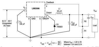
O Some connections have to be sort with thick wires. In PCB designs the ground has to be a copper flooded area. Many implementations on a breadboard will fail!!
