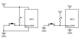
the ground. We use to keep that in drawing also as much as we can, (left) placing VCC upwards and ground downwards. From
