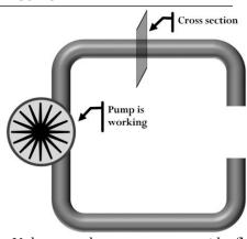
In our electronic—hydraulic analogy, our fluid needs a closed loop hose to flow since the pump in our previous shape only recycles the fluid inside our hose. A wire that makes a closed loop is called circuit or closed circuit. Open circuits have zero current flowing through them.
