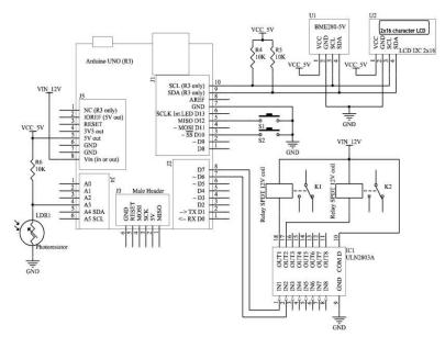
It should be powered by the Arduino's DC socket with a 12VDC supply. That is intentional for driving our relays coils and for understanding better the NPN or open drain switching capabilities. Taken from left to the right:
