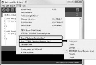
(Board: "Arduino/Genuino Uno"). Genuino is a name coined by the Arduino team later but everybody is still using their original one, Arduino. Then select the correct Port, which is the correct Serial Port. You should see a list of serial ports. If none is advising that an Arduino Uno is connected to it, you have to try each of them. After selecting a port, try "Get Board Info". If you have selected the right
