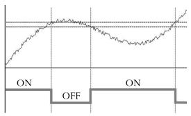
On the left we see what the two first 2 ifs do. The feature is called hysteresis. It solves the problem of switching the K1 relay on and off rapidly while the
