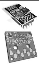
When we say "electronic board" we mean Printed Circuit Board (PCB) with electronic components mounted on it. This is the top way we may construct our circuits. The components are all soldered as we will see in the next paragraph. PCBs are a flat, insulating and heat resistant material, with patterns made of copper foil on its surfaces that connect component pins together. So instead of wires we have a rigid body with conductive tracks running in complex point to point. We will present them
