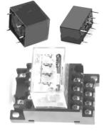
isolated from the coil's poles. Relays come with most kinds of two position switches (SPST, SPDT, 3P2T, 4P2T...). Their main specifications is the switch's conducts maximum current (usual is around 2A-10A) and the coil's voltage needed to activate (3V to 220V). They are mounted on circuit boards (PCBs) or on sockets (base) providing terminals to easily screw cables on them.
