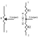
consume (P=V\*I) may vary according to the position they are set (e.g. go too high in very low Ohms settings). Another interesting thing about them is that they provide 3 pins, working as you can see on the left, either as a variable resistor if pins 1 & 3 or 2 & 3 are used, or as a voltage divider if all 3
