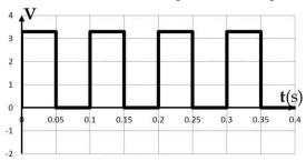
Diagrams where the input variable (horizontal axis) is time show how something evolves — changes. You may meet the term "transient response" for this.
