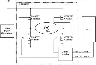
"H", in our example turning ON "1" and "4" will spin the motor to one direction , turning ON "2" and "3" will spin the motor to the other, non or "1" and "3" or "2" and "4" ON will stop it.
