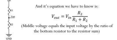
They connect their "outer" ends to a voltage, their middle point is a fraction of the "outer" or supplying voltage. This is going to be a guy we will usually hang out with in electronics designs, so let's meet him better.
