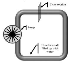
will only talk about metals, the electricity conductors. In metals as said, some of their atoms' electrons move freely. Let's imagine a metal wire like a hose inside which, instead of water, electrons flow, but like water they make an uncompressed fluid. Also imagine that all of the hose/wire is filled up totally
