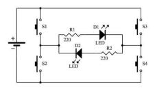
6. When both S1 and S4 are pressed D1 shines. When both S2 and S3 are pressed D2 shines. You should not press simultaneously S1 and S2 or S3 and S4 of course
