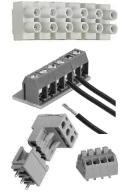
a way to connect / disconnect a cable stripped at its end to another cable or a PCB or a breadboard without soldering / disordering. On the left, from top to bottom, we see some representative terminals: Cable to cable screw terminals, PCB mounted screw terminals, two pieces pluggable type (one piece is permanently mounted on a PCB, the other carrying the cables is detachable) and spring loaded type where instead of using screws we only have to press inwards a spring
