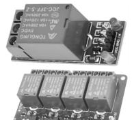
pin needs the help of a MOSFET or a BJT transistor. It also needs a diode in a tricky connection to protect our active component. It is handy and money saving to use relays with all this circuitry included, ready to accept GPIO signals costing around 0.5\$ per relay, each providing an SPDT switch holding 10Amps. Another variant of relays are the solid state relays or SSRs which are fully
