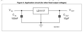
That is how almost all regulators are used. They require 2 capacitors placed close to them for charge reservoirs, one at the input and one at the output. Other specification highlights are:
