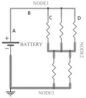
resistor's symbol. On the left we have a circuit with 3 nodes. No matter how long wires we use in our schematic e.g. making the simplest path or making a maze with the wires of one node, it is still the same one node, all pins it connects are connected the same way, as if they are connected on a single point. The reason this happens is that a zero resistance
