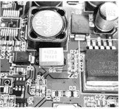
the game to dominate more than the 95% of electronic components. 99% at least of all MCUs in the last 20 years are SMD, so are the most important ICs. SMDs do not have wires, but only very sort pins. They are designed to be soldered on the same side of the PCB — on the surface
