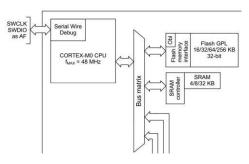
At the heart we find the computer. A CPU (Central Processing Unit) or "core" where the commands of our program are executed, memory of permanent storage type and volatile type. Permanent
