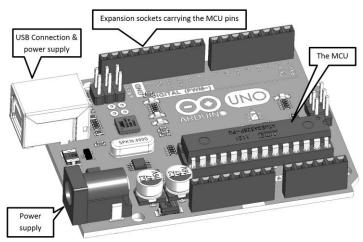
An Arduino board offers an easier way to use an MCU rather than having the MCU chip alone, namely:
