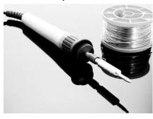
you might and you might not get a minimum burn. Soldering Irons are devices which heat a tip at the right temperature to melt solder wire and their tip is at the right geometry to interact with electronic components of some size. It requires
