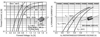
1A diodes are medium in size, smallest are around 200mA maximum current, biggest practical are around 5A. Diagrams above show current over 1A that they can handle only on sort durations. Note the logarithmic vertical axis. Now notice the main difference between the real and the ideal diodes. Instead of "turning on" at 0V or at 0.000001V they start to act like a sort circuit after a voltage called  $V_F$  or  $V_{FORWARD}$ . If current of 200mA flows on the circuit on
