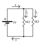
branch into  $I_1$  and  $I_2$  ( $I=I_1+I_2$ ). Since there is a narrow path and next to it in parallel another narrow path, the current flows easier now than having one narrow path only. In our case **the total resistance is the half** of 1.2K (it equals 0.6K). Current I is therefore I = 3V/600Ohm = 0.005A (or 5mA) (half resistance makes double
