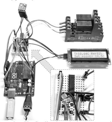
We used a small breadboard here that just fitted, so components and wires on it had been a little dense. The circuit worked well, the advantage of this method is that we can make that spaghetti circuit in less than 20 minutes, so it is a nice way to check our schematic design (not in all cases though, like DC/DC regulators, power circuits, sensitive signals circuits and SMD components).
